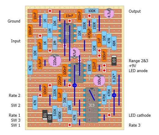
IC1: TL072 Range: A50K Range 1 to ground IC2: TDA7052A Rate: B50K
