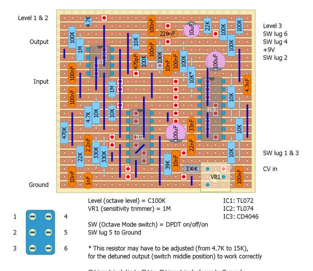
CV input jack tip to CV in. CV input jack sleeve to Ground
