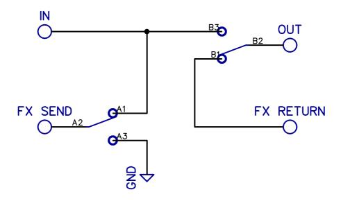
Note that in bypass, the FX input is grounded
