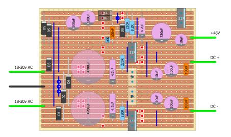
5K are multiturn trimmers. Adjust for +/- 17v
