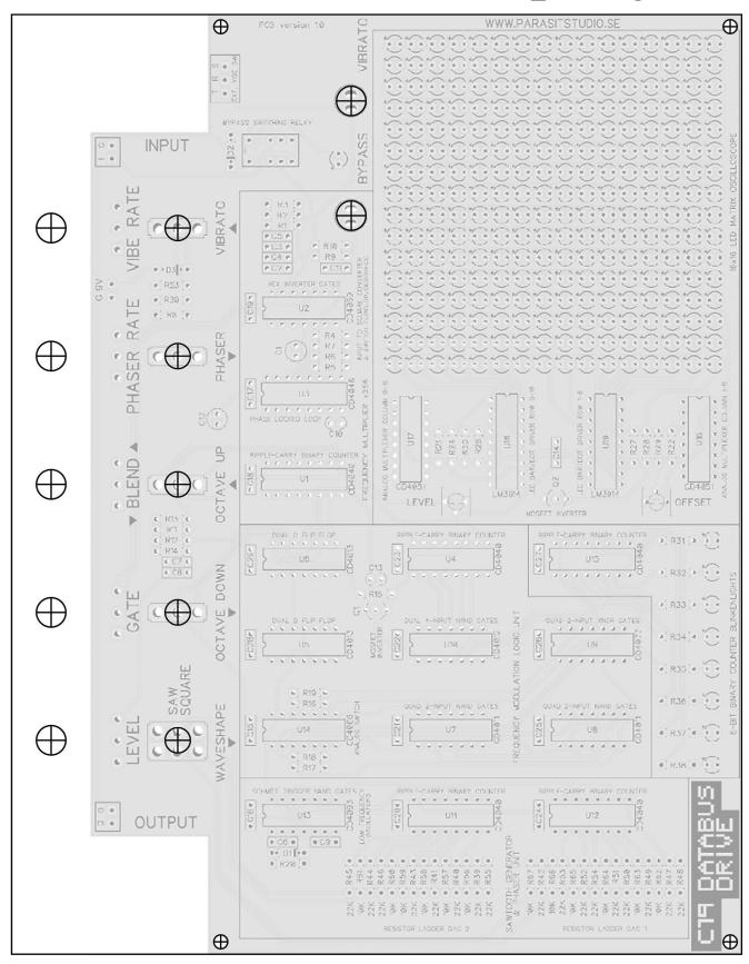
Make sure your printer isn't doing any scaling. Measure and confirm before drilling. Hold the template against the PCB to me sure that it's the right size. Drill holes for the input/output jacks and DC jack to your own preference.
