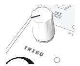
The TRIGG knob needs to be turned up to get any sound out of the pedal. It controls the input level so that it detect when you play a note / pluck the string.
