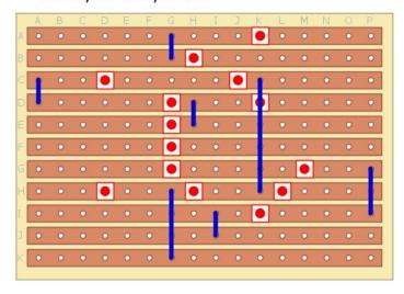
This layout is missing a 47uF cap between +9V / ground - Solder it directly to the DC jack
